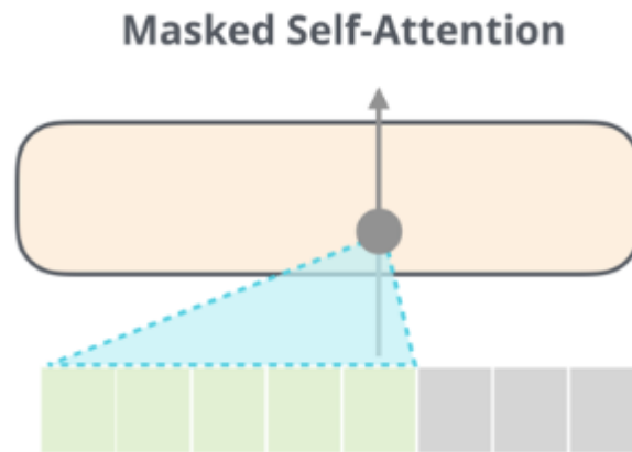
Figure 2.22 Mask Self-Attention's Working
