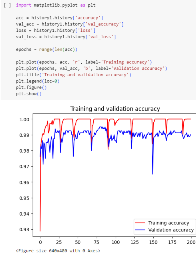
Figure 4.5: Graphs depicting the growth of Training accuracy (in red) and Validation accuracy (in blue) as the number of epochs increases on the MALIMG dataset.
